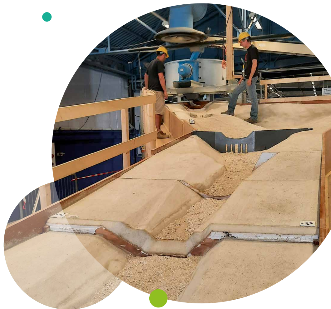
CNR uses a physical model to assess the operation and possible adaptations of the sediment regulation structure of the Manival (Isère), one of the most active and developed torrents of the Alps.
