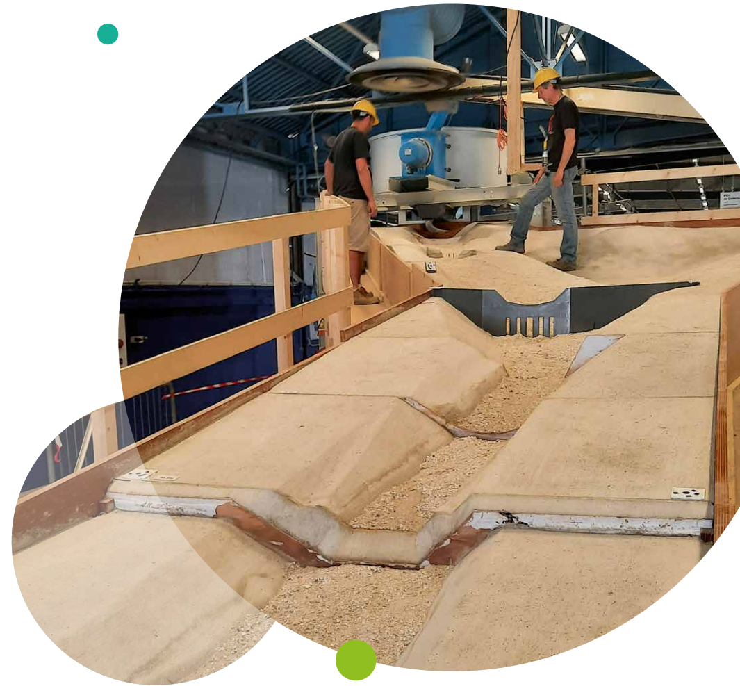
CNR uses a physical model to assess the operation and possible adaptations of the sediment regulation structure of the Manival (Isère), one of the most active and developed torrents of the Alps.
