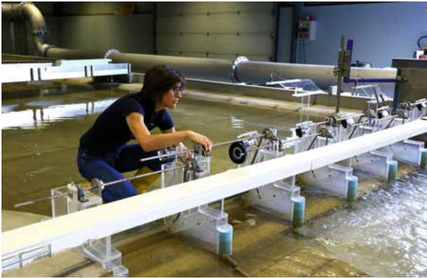
Study using a physical model to understand erosion phenomena downstream of Donzère dam
